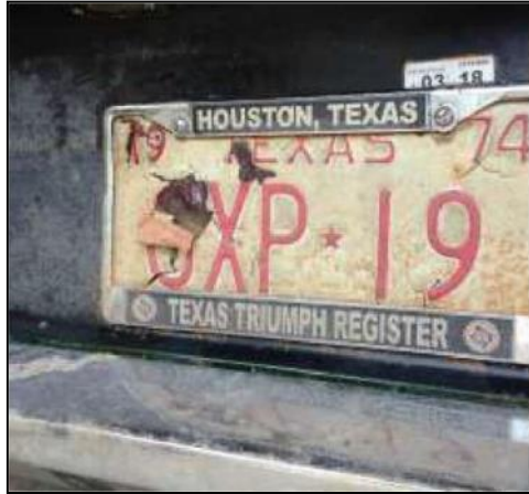
What 13 days of flood water does to a restored license plate – from Len and Marti Myers’ totally submerged TR6 now in restoration
