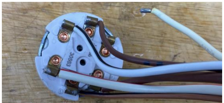
New Lucas switch with unattached #3 run wire
