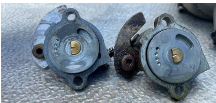
Dirty and Clean Starter Boxes
